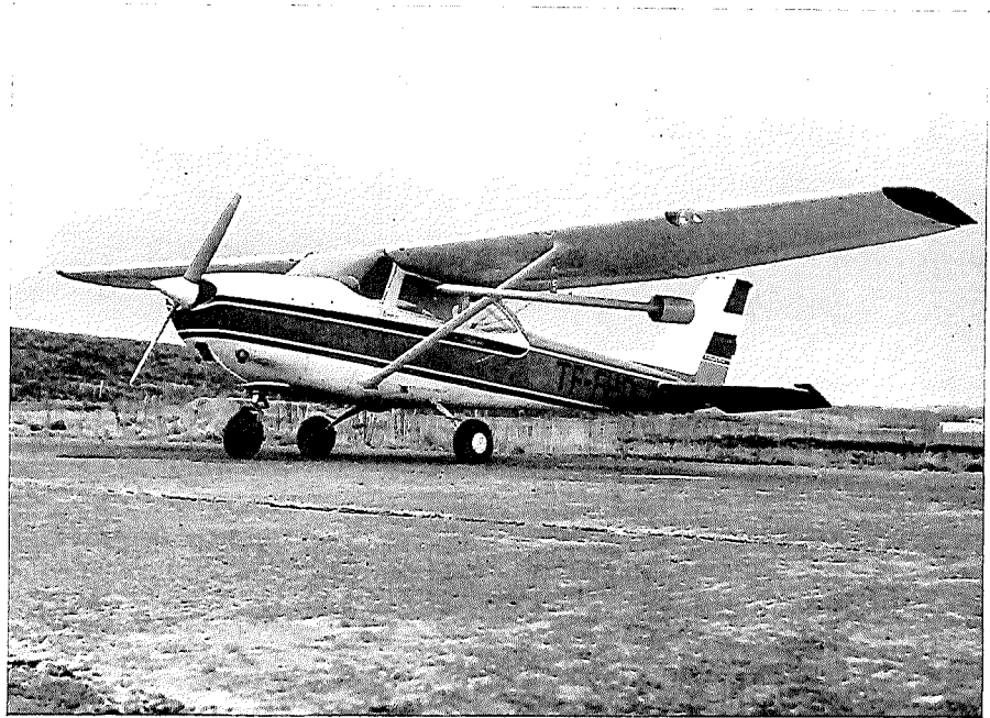
Fig. 1. The survey plane with the magnetometer hanging from its wing.
