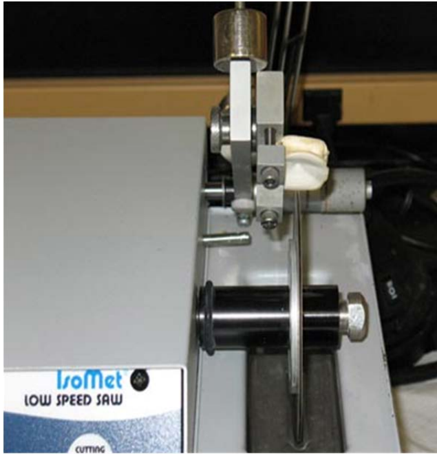
Figure 3. Preparing a section of a vertebra with an IsoMet saw.
