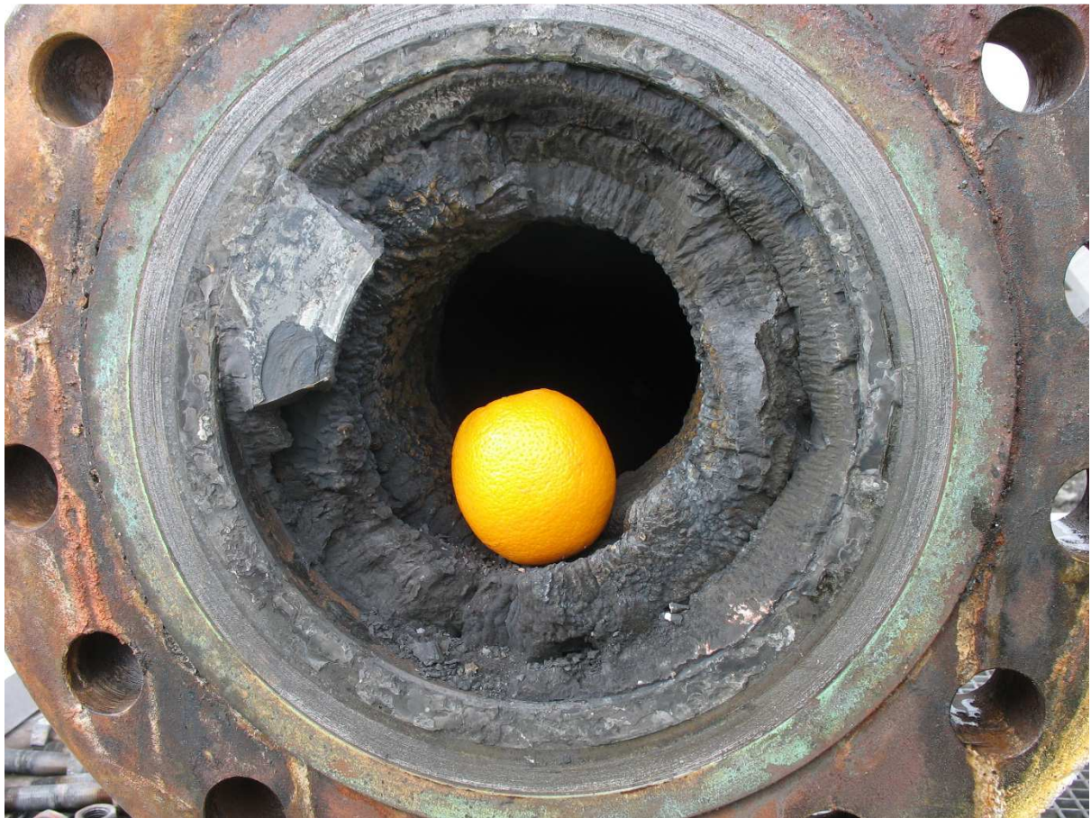
Figure 2. Scale precipitated in a pipe from well RN-22. The scale is formed in one year from 2006-2007. An orange has been placed for size comparison [6].
